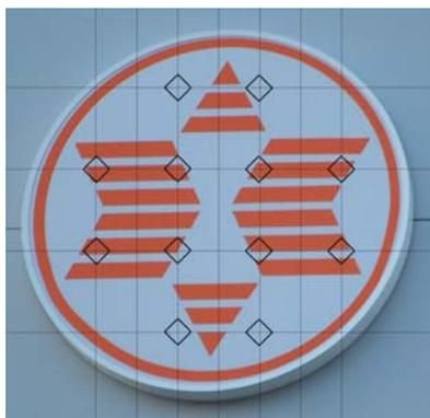
Expert 1500 mm diameter sky sign using 12 QL4 QuarterLites, as shown on the overlay above.
